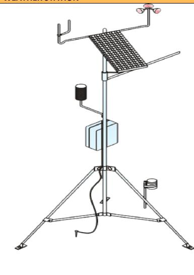
Our weather stations are known for their precision measurements rugged construction. It has wide operating temperature range and low power consumption. The standard weather station consists of a weather proof enclosure which contains the data logger and power supply and come complete with solar panel tripod stand and basic range of sensors.
